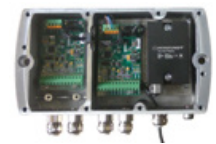
3 Inclinometer in connection box
